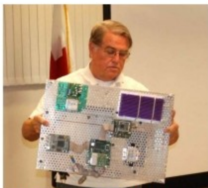
Robbie KB6CJZ showed his progress building a DigitalATV repeater station (1.2 GHz up / 3.4 GHz down) (photo by W6HHC)
