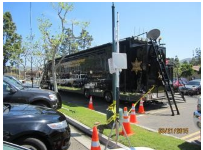
Figure 11 2.4Ghz NanoStation Station D and 5Ghz Rocket Station E with dual- channel flat panel antenna receiving video streams from two strings of ipCams across the San Juan Capistrano downtown parade route
